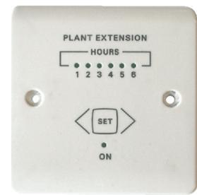
The TPEXT1 touch sensitive Plant Extension Timer is designed to extend the normal period run time of a system for a selected time. The TPEXT1 Extension Timer operates a set of normally open volt free contacts and is available for 24V AC and 240V AC operation with build options for 0-3, 0-6, 0-12 and 0-18 hours.
